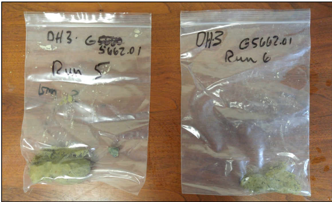
Soil (clay) was recovered in coring samples NQ-5 & NQ-6.
